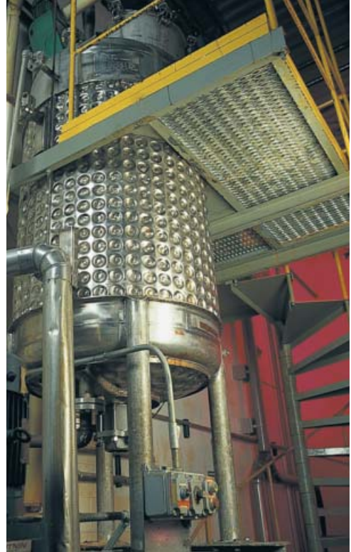
One of many reactors used at Essential Industries in the production of polymers.
