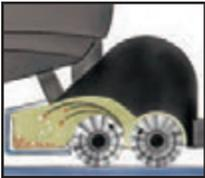
The CT160 Cylindrical is equipped with 30" dual counter rotating brushes to sweep, wash, and dry in just one pass. Ideal for grouted tile and warehouse floors.
