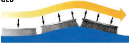
A uniform scrubbing apparatus guaranteed by the spring-activated floating head, which adapts instantly to even the most irregular surfaces.
